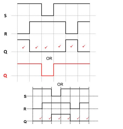
**NOTE:** If SET and RESET are both "1" the principle of NO CHANGE for the inputs at both 1's should be followed.
