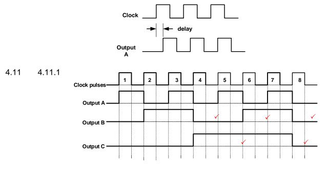
4.11.2 The purpose of the AND gate is to prevent  $FF_2$  from producing an incorrect reading on the second clock pulse  $\checkmark$  when  $FF_0$  and  $FF_1$  are both high (3<sub>10</sub> or 11<sub>2</sub>)  $\checkmark$  and the next pulse must produce a 4<sub>10</sub> (100<sub>2</sub>).
